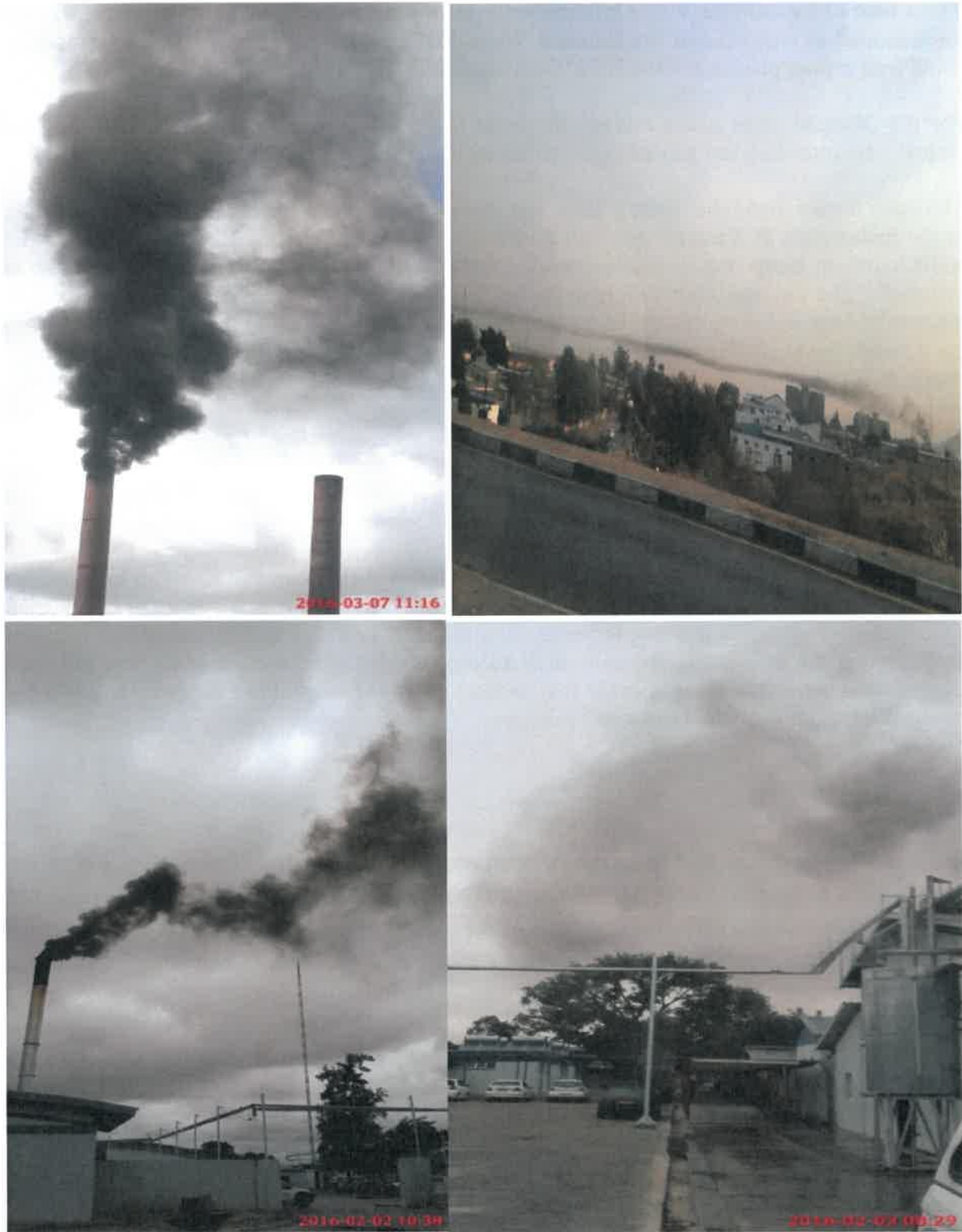
Picture 21: Emission of thick dark smoke from the chimneys at the incinerators
