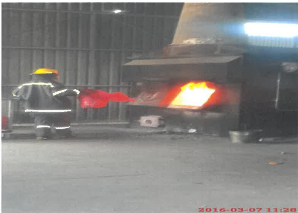
Picture 22: Manual loading into a Combustion Chamber
